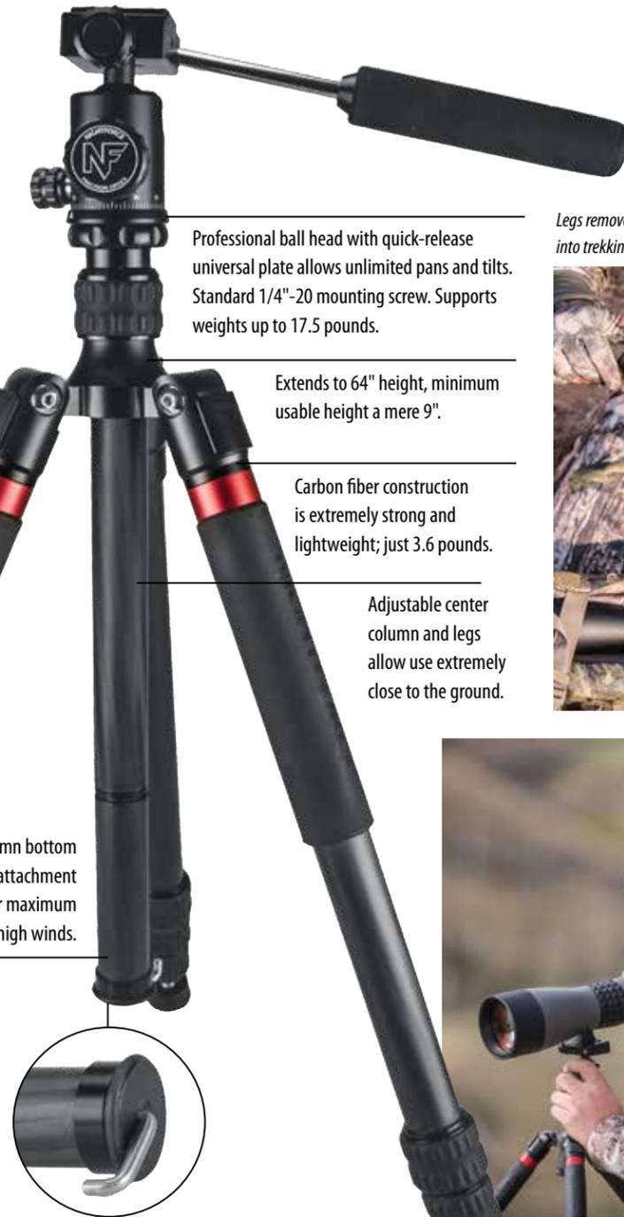
Professional ball head with quick-release universal plate allows unlimited pans and tilts. Standard 1/4"-20 mounting screw. Supports weights up to 17.5 pounds.
