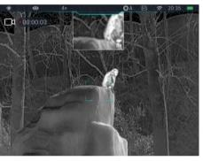
main image is enlarged by  $1\times$ ,  $2\times$ ,  $3\times$ , or  $4\times$ , the image in the PIP window will be enlarged by  $2\times$ ,  $4\times$ ,  $6\times$ , or  $8\times$ respectively.
