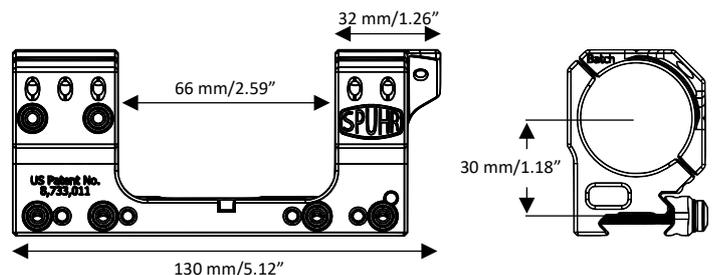
The mounts are machined from billet 7000 series aluminum and all aluminum parts are hardcoat anodized. The Torx 20 ring and clamping screws are zinc-nickel coated for corrosion resistance and come pre-waxed from the factory to ensure proper torque values.
