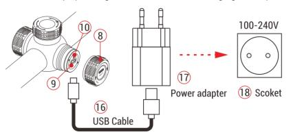
Note: The USB port can only be used for charging the built-in battery pack
