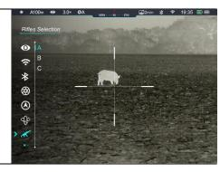
Please select a zeroing profile and set the zeroing distance before carrying out any zeroing operation.
