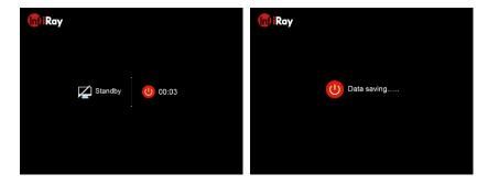
Releasing the button during the countdown, the device will enter the standby mode. Press the **Power button (5)** again to wake up the device.
