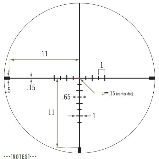
Subtensions are measured in MRAD and correspond to the highest magnification.  $\varnothing$ =Diameter
