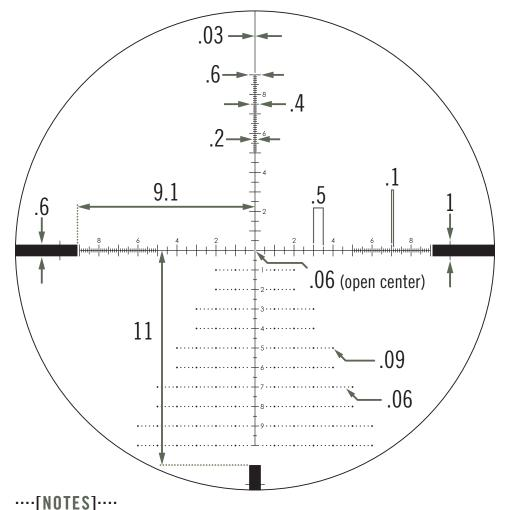
Subtensions are measured in MRAD and remain constant at all magnifications.
