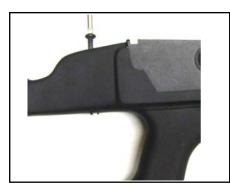
Insert the original tang screw into the pre-drilled hole on the fiberforce stock, and then tighten using a phillips head screwdriver as seen in Figure 6.
