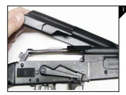
Note: Trigger assembly must be modified to the forward position for the installation of ATI's Fiberforce Pacakges. Disassemble the Saiga using your owners manual. Begin by removing the receiver cover from your Saiga as seen in Figure 1.
