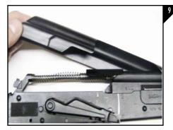
Reinstall the receiver cover as seen in Figure 9 to complete your installation.
