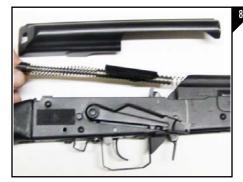
Reinstall the recoil spring as seen in Figure 8.
