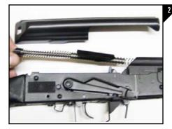
Remove the recoil spring from the shotgun as seen in Figure 2. Place both the recoil sping and the receiver cover aside for later installation.
