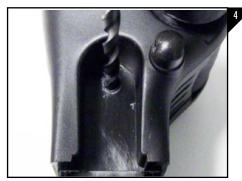
Next, remove the pivot assembly and start drilling a pilot hole in the center of the marked hole with a 1/16" starter drill bit as seen in Figure 4.
