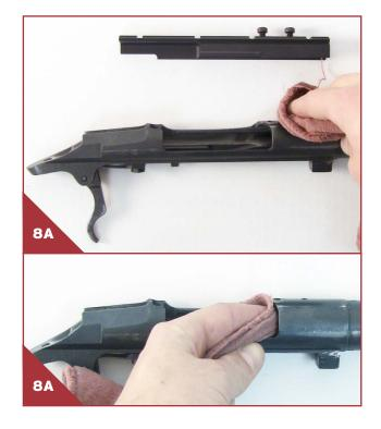
Set the scope mount in place, install and tighten screws the provided  $10-32 \times 1/2$ " Slotted Flat Head Screw (Thread lock is recommended.) Check screws to be sure they do not protrude below the inner surface of the receiver as seen in Figure 9.
