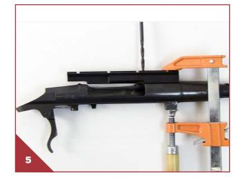
With the mount still clamped, use the supplied (smaller) #21 drill bit as seen in Figure 6, drill slowly so as not to burr the inside of the receiver below the hole. (It is recommended to use cutting oil during the drilling process.)
