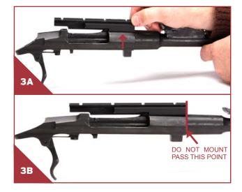
Install the scope mount in the proper position as seen in Figure 4A. If you attempt to install the mount in an improper location or on the barrel as seen in Figure 4B, damage to the property, injury or death will occur.
