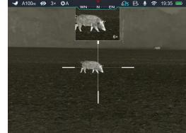
magnification of the main image is  $4\times$ ,  $8\times$ ,  $12\times$ ,  $16\times$ , the corresponding magnification of the PIP image is  $8\times$ ,  $16\times$ ,  $24\times$ ,  $32\times$ .
