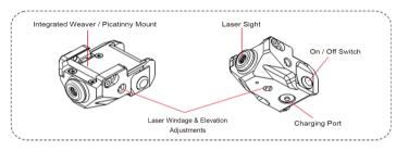
Simply click On/Off switch to turn the unit on or off.
